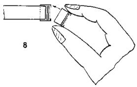
Step #8: Bring tilted mounting ring to the light pipe (so scintillator does not fall out) and slip directly onto the end of the light pipe.
