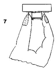
Step #7: Hold SEM mounting ring tight and turn all upside down. Scintillator should fall into the SEM mounting ring.
