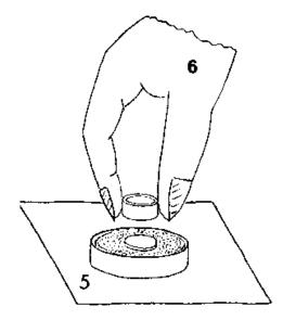
Step #5: Remove cover glass with care. The scintillator is left in its position with the powder coated surface facing "up". **Warning**: *Do not touch the powder surface!*
