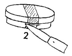
Step #2: Cut the adhesive tape on both sides with s sharp knife or razor blade.
